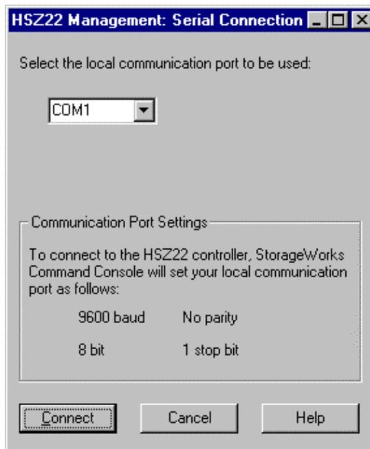
Figure 3-4. HSZ22 Management Serial Connection dialog box for Storage window
