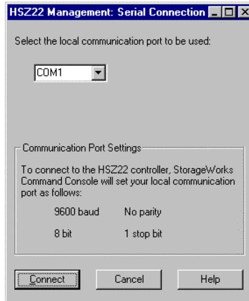
Figure 2-4. Establishing a connection to the top controller
