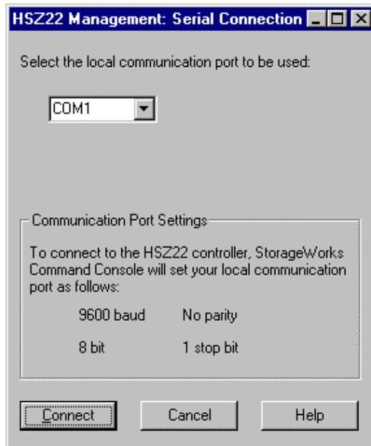
Figure 3-5. Establishing a serial connection to the top controller
