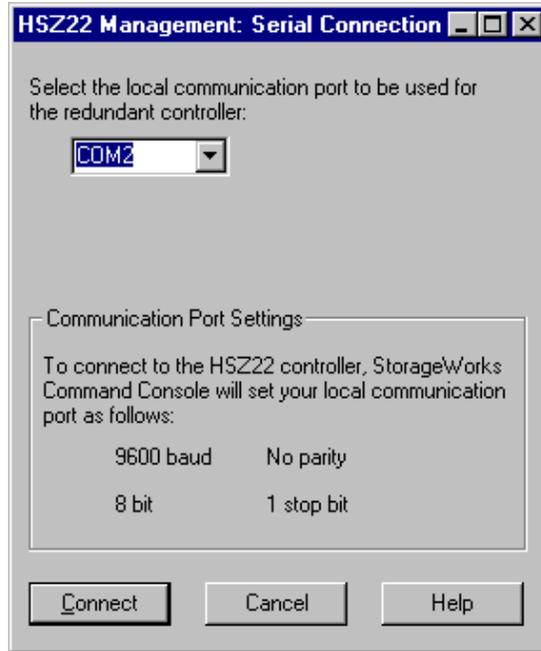
Figure 3-6. Establishing a serial connection to the second (redundant) controller
